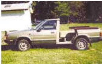
the cab behind the front seat and cut a hole in the rear of the cab with a chop saw so I could install a Plexiglas window. A shop-built 4 by 6-ft. wooden box slips in the back of the vehicle between the wheel wells. It's ideal for holding fence-fixing tools, rocks, sticks, etc. Cost only about \$100, including new battery, water pump and oil seal.
