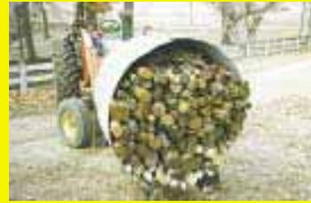
laid the hog feeder on its side and bolted it to the railroad tie and used 2 by 6's on the side of the tines to hold the feeder in place.
