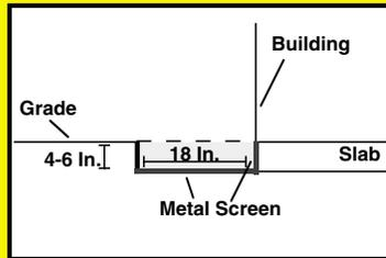
22-in. wide strip of metal screen, or hardware cloth. Lay the screen in the trench and then cover with dirt to grade. Rats like to dig right next to the foundation so when they hit the screening they do not know enough to move back a couple feet.
