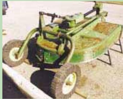
Pto-powered rotary flail mower was converted to giant "weed eater" by replacing the blades with lengths of log chain.
