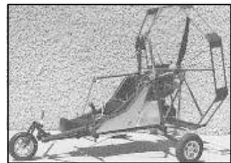
The machine is powered by a 52 hp twin-ignition Rotax engine and 5 1/2-ft. propeller. The back seat was removed to install a 30-gal. tank and 35-ft. spray boom equipped with four electronic rotary disc nozzles that apply chemicals at ultra-low rates. It features a 520 sq. ft. parachute and is capable of carrying a 550-lb. payload.
