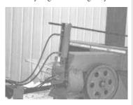
thrower control for Deere small square ejection balers. These balers come with a steel rod that you have to manually rotate in order to adjust the bale's throwing distance. To change the setting you have to reach behind from the tractor cab and rotate the rod, which is awkward to do. My thrower control uses the tractor's hydraulies to rotate the rod and is activated by a valve in the cab.
