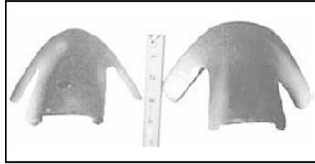
**Cultivator blade on left was used as purchased. Blade on right was cryogenically treated. Blades were attached next to each other on the same cultivator and were used to cultivate 3,600 acres.**
