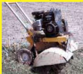
solve the problem, I cut a 5-gal. plastic pail in half and bolted the two halves onto the tiller frame over the top of the blades. Now the churning dirt stays inside the plastic covers and, instead of throwing lumps out, it chews them right up and leaves the dirt real fine so I can till right next to plants. The metal brackets I made let me adjust the covers up or down. **(Robert Sexton, Rt. 1, Box 2A, Millville, Minn. 55957 ph 507 798-2492)**
