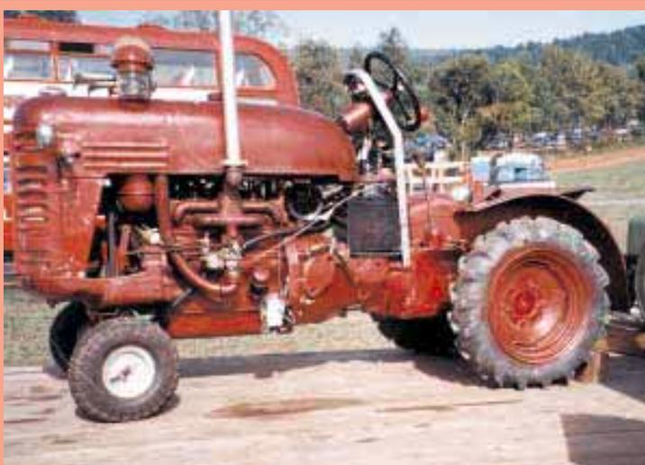
I thought your readers might enjoy this photo of my modified Farmall tractor. I call it my Farmall Cub Jr. It's 90 percent IH and 10 percent other stuff. I cut 18 in. out of the tractor's main housing and 11 in. out of the hood. I replaced the original front axle with a wide front axle which I bought at a flea market. The rear axle
