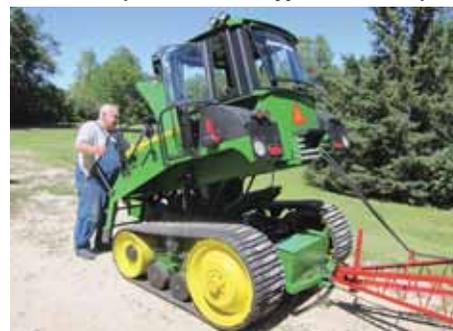
The back end of the tractor lifts up, providing access to all the hydraulic valves and gearing underneath the cab.
