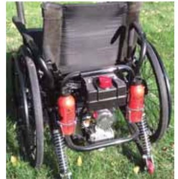
**Engine mounts on subframe below and behind wheelchair seat.**
