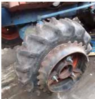
**David Simpler’s Kubota tractor was light on the front end, so he mounted two 16-in. dia., cast iron Brillion cultipacker wheels at 25 lbs. apiece on the front rims.**
