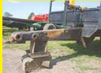
I saw this trailer at an auction and immediately thought of FARM SHOW. It was home-built in Scotland from various odds and ends. What caught my eye was the drawbar. It's made from the "dipper" end of an old backhoe – the section of
