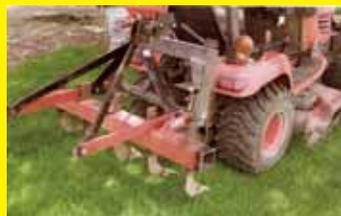
I made a "ripper" out of a box blade. It's about 5 ft. wide, just the width of the tractor. I left the braces on top and back for strength. It fits on my 23 hp. Kubota tractor's 3-pt. hitch. Lets me plow my garden in about a third of the time that it used to take me with a 2-bottom plow. The teeth are adjustable for depth. **(Bernard Marvel, RR 1, Box 44, Browning, Ill. 62624)**
