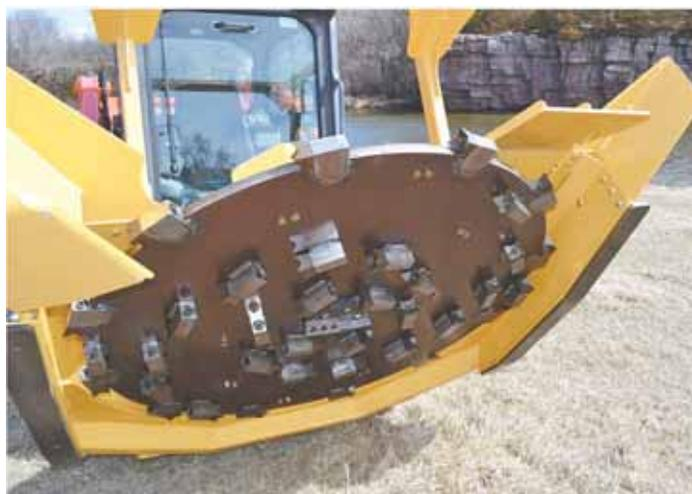
The 5-ft. wide Forestry Head can saw through up to 24-in. dia. trees and mulch 6-in. trees. It’s fitted with 24 planer knives mounted randomly on dish.
