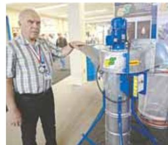
Polish seed cleaner uses centrifugal cleaning action to separate grain from trash.
