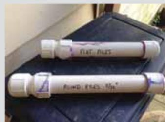
"To solve the problem I decided to store the files inside big diameter soda straws that I then place inside pvc tubes. The straws keep the files from bouncing around and rubbing against each other and becoming dull. I can store up to a dozen 5/32-in. round files inside a 1 1/2-in. dia. tube. I place a silicon bead pouch (the kind you often find in shipping boxes) at the bottom of the tube in order to draw away any moisture.
