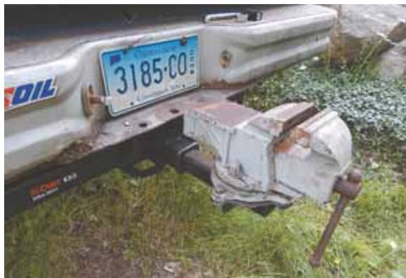
Bishop bolted a steel plate onto a vise and then welded the plate to a length of 2-in. sq. tubing, which fits into vehicle's receiver hitch.
