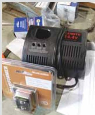
**Richard Rogers, Bentley, La.:** "The charger went bad on my Alemite 14.4-volt battery-powered grease gun due to a bad transformer. A replacement charger from the company would have cost about \$150. Instead, I replaced the bad transformer with a 16-volt doorbell transformer that I bought at Home Depot for \$11.
