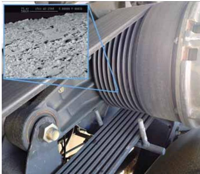
Photo shows pulley treated with Vulcan Grip on a Claas 980 self-propelled forage harvester. Vulcan Grip’s ultra-hard microtexture (inset) resembles an asphalt road surface under a microscope.
