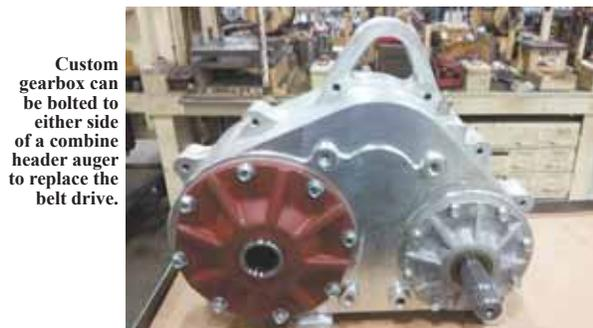
Custom gearbox can be bolted to either side of a combine header auger to replace the belt drive.
