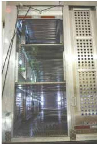
Prototype semi trailer has 2 decks that can be hydraulically raised into place while loaded. Photo above shows decks in lifted position. Photo below shows lift decks down.
