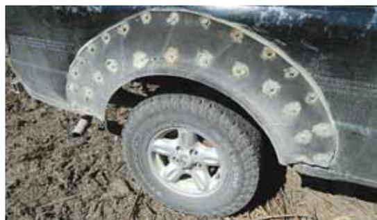
Dave Gilbertson fitted his rusted-out pickup with "tire fenders" that he made by cutting the sidewalls off small tractor tires.
