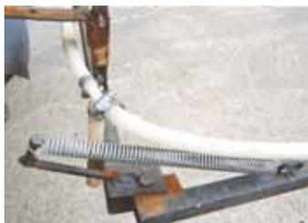
Each boom wing is held in place by a 7-in. long spring fastened to a metal arm.
