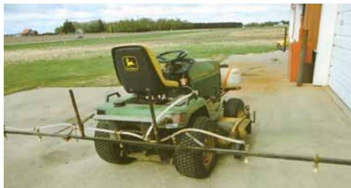
Lester Adelman's 3-section sprayer has a 14-gal. tank that mounts on front of his Deere 445 riding mower, and a 10-ft. breakaway boom on back.
