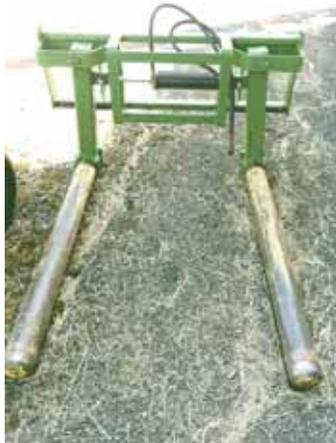
Equipped with rolling pipes instead of grabbers, Allen Pansegrau's big round bale lifter avoids messing up the plastic on silage bales.
