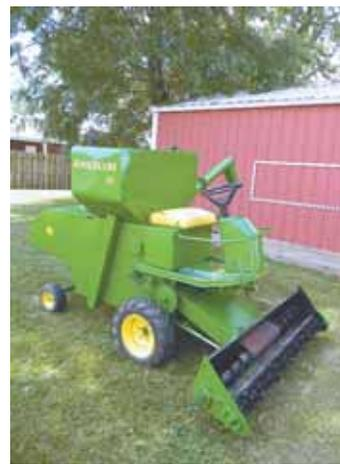
Combine's 5-ft. header is fitted with three 21-in. reel mowers mounted side-by-side.
