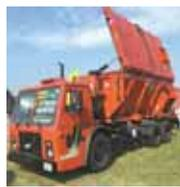
**Truck-Mounted Side Discharge Manure Spreader** - Ranging in size from 2,600 to 4,200 bu., H&S Manufacturing's new spreaders can handle liquid or solids. A 200 hp. hydraulic pump with 70 gpm flow provides the spreading power. Can be equipped with an optional hydraulic-operated lid. ([www.hsmfgco.com](http://www.hsmfgco.com); ph 715 387-3414)
