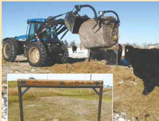
Inventor Dick Schirado uses a grapple fork to pick up bales and slides it over top of blade to cut through net wrap.
