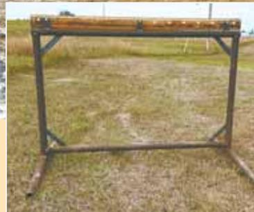
Home-built net wrap cutter consists of a 7-ft. steel blade mounted on a metal stand.
