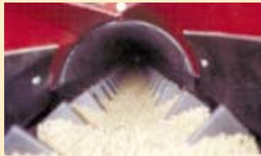
Tube Conveyor With Cleated Belt
