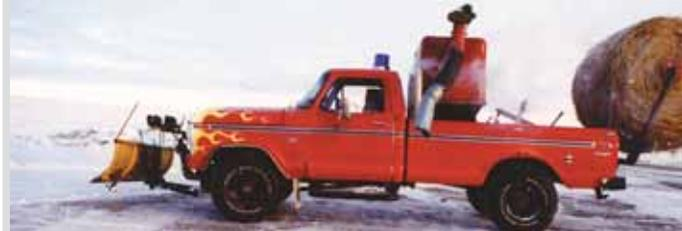
Converted Ford F-250 is equipped with a round bale unroller and a modified feed unloading bin on back, and a winch-controlled snow blade on front.
