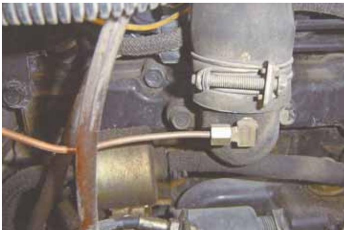
He drilled a hole in the manifold, tapped it, and installed an elbow. Then he ran a length of copper tubing to it through the tractor's side panel.
