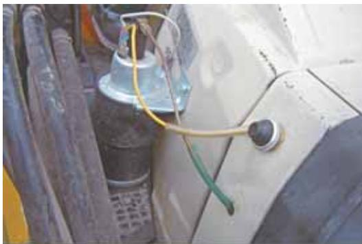
Richard Mountcastle replaced the glow plug starting system on his Cub Cadet diesel utility tractor with one designed for a Case IH tractor. He mounted the injection system and a push button on the right side of the dash.
