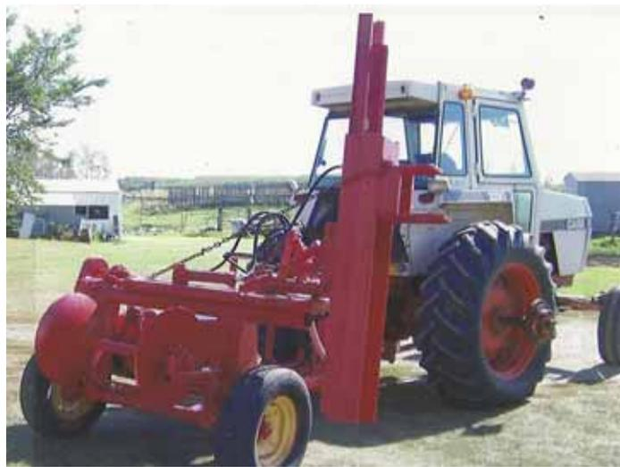
Tractor's hydraulics operate the post pounder, and the pto operates a gearbox that chain-drives the wire roller.
