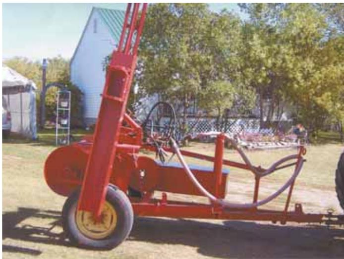
Delbert Logan welded a Shaver post pounder to one side of a Massey Harris pull-type swather frame, then added a home-built, 3 1/2-ft. wide wire roller on back.
