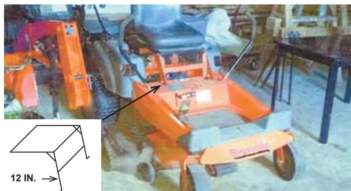
Howard Aul wanted to sit higher on his Husqvarna zero turn mower, so he made a metal bracket that raised the seat about 12 in. and shifted it back over the engine.
