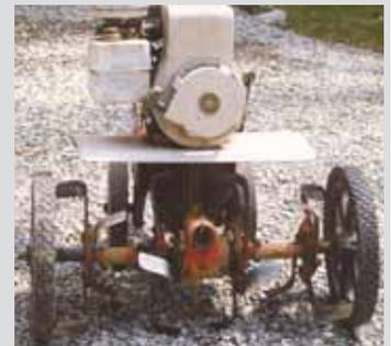
Add-on wheels propel rototiller forward and take all the work out of driving it around.
