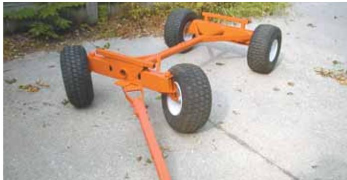
Nichols started with the front axle and wheels off an MTD garden tractor to build this mini wagon running gear. It looks and works like an actual farm wagon running gear.
