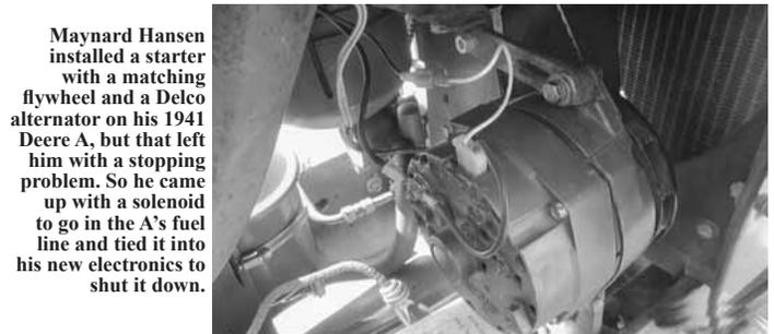
**Maynard Hansen installed a starter with a matching flywheel and a Delco alternator on his 1941 Deere A, but that left him with a stopping problem. So he came up with a solenoid to go in the A’s fuel line and tied it into his new electronics to shut it down.**
