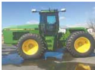
**This Deere 8760 has been retrofitted with AutoDrive which includes a laser positioning system, sonar perimeter sensing, and cameras to gauge distance, velocity, and direction.**
