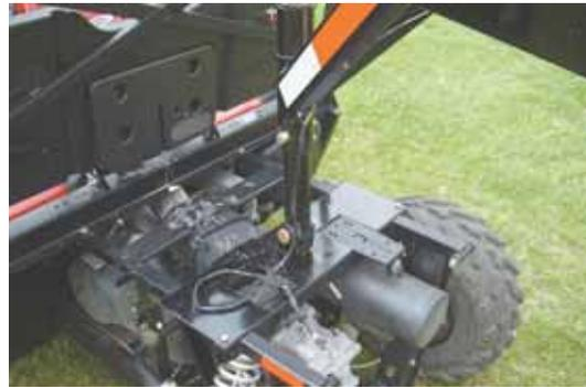
The vertical post for the gooseneck was fabricated from 18-in. long, 3-in. dia. pipe. Another pipe inside makes it easy to adjust the height.
