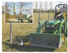
Hydraulic-powered cutter attaches to loader bucket.
