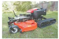
Remote-controlled tracked mower can be operated by a handheld transmitter from up to 300 ft. away. The low center of gravity makes it safe to use on steep hillsides.
