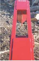
Log splitter is built from two pieces of channel iron mounted back to back, with an 8 by 24-in. window" in between. The window design lets Trelstad see what he's doing and is also stronger" than a single I-beam.
