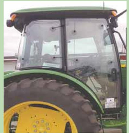
Tractor Guard window protectors are designed to protect your tractor’s windows and mirrors from flying rocks and trash.
