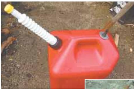
Brent Gill came up with his own vent for plastic fuel cans. "With the core valve removed, it's easy to fill a tank because air rushes in through the valve when the cap is removed," he says.
