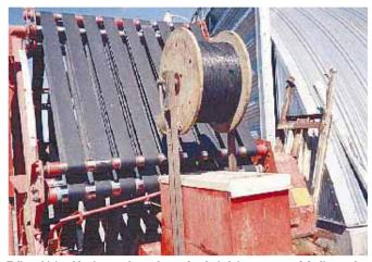
Falkowski ties old twine together end-to-end and winds it up on empty 2-ft. dia. wooden welding wire spools. Twine feeds into baler just like it would out of twine box.
