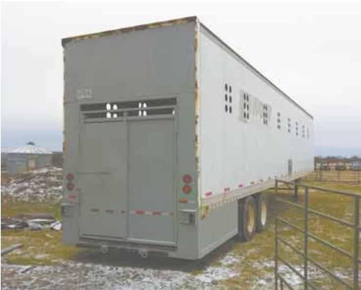
**Gary Bueckert saved the cost of a new cattle hauler by converting a semi trailer into this ground loading model. The former 53-ft. van carries about 30 head at a time.**
