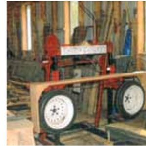
In 2010 Reeks designed his latest new sawmill, the Thriftwood. It's powered by a single phase 220-V motor. No fumes so it can be used inside.
