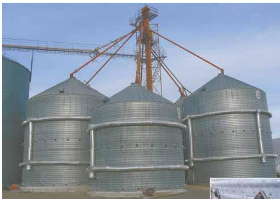
Ben Casper’s Sectional Drying System uses fans to push fresh air through specially vented bins to dry the crop. No heat is needed. As air passes into the grain it picks up moisture that flows into exhaust tubes (right) that exit through the bin’s sides.
