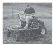
Tom DuFresne, Grant, Minn.: "I've used my Schweiss zero turn mower for 12 years with almost no problems (Schweiss Welding, www.schweisswelding.com; ph 507 426-7828). Most of the parts are standard off-the-shelf components so you can buy them anywhere. My mower has a 72-in. deck and steers with a single joy stick so it's very maneuverable and easy to use. I hope I never have to mow with anything else."
