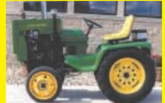
I always wanted a garden tractor equipped with a Deere 2-cyl. engine, so recently I mounted an LUC engine off a Deere 12-A combine in a Deere 318 garden tractor. It's chain-driven and has a hydrostatic transmission. (*Norman Kielsmeier, Rudd, Iowa 50471 ph 641 395-2668*)
