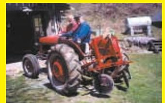
I built this 3-pt. mounted "lay-off plow" to plant potatoes in my garden and use my 1950 Ferguson 85 hp tractor to pull it. The unit consists of two 16-in. dia. discs mounted on a frame that's made from 3/8-in. thick, 2 1/2-in. angle iron. The discs are spaced 1 1/2 ft. apart and hill up the soil about 6 in. high.
