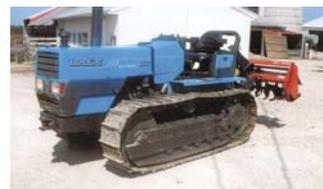
**Mike Zimmerman, Versailles, Mo.:** He’s pleased with his 1999 **Landini 65F** ag crawler tractor. “I bought it used in 2006 with only 1,600 hours. The tractor has a 65 hp Perkins engine with a 16-speed transmission, 3 pt. hitch, pto, double hydraulics, and hydraulic steering.
