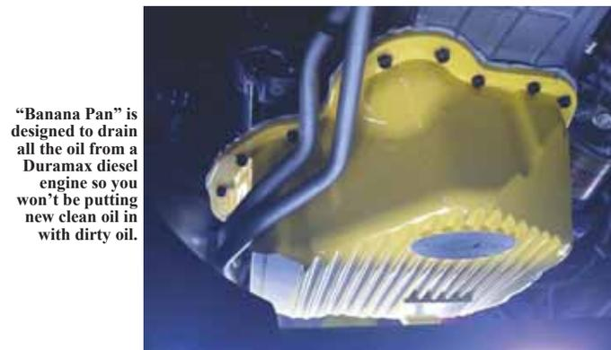
"Banana Pan" is designed to drain all the oil from a Duramax diesel engine so you won't be putting new clean oil in with dirty oil.
