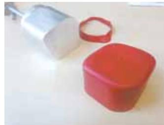
Deere never made a cover for an exposed circuit block on its 5425 tractor, so Randy Smith made his own. Photos show mold with new plastic cover (left) and cover installed over fuse block.
