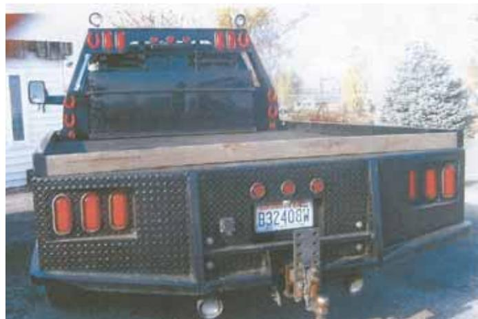
Alan Heilman fitted his Dodge 3500 1-ton dually pickup with a flatbed, that rests on two 1-in. thick steel bars.
