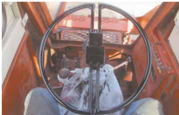
When Glenn Buxengard reversed his Allis Chalmers loader tractor to mount a cab on it, he could hardly get in to sit down. So he cut the tractor's steering wheel in half and added a folding mechanism.
