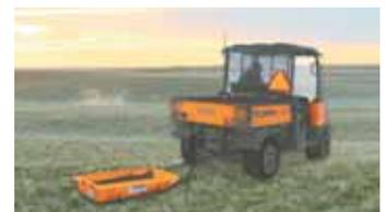
Runners built into heavy-duty plastic sled allow it to slide easily along the ground.
