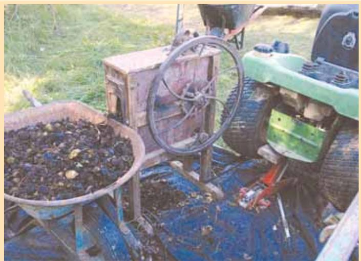
John Kocur used one of the wheels on a riding mower to friction-drive an old hand-cranked corn sheller. “It really works slick to crack walnuts,” he says.
