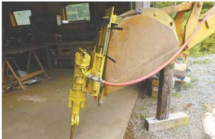
Jackhammer bolts onto backhoe's bucket and operates off a compressor.
