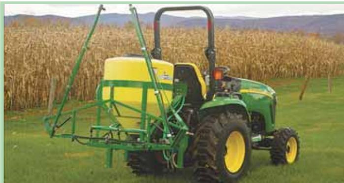
Alvin Wittmer's 3-pt. mounted sprayer comes with a 12 or 18-ft. boom that can be extended in 18 or 36-in. increments, and filled with an 80 or 35-gal. tank.
