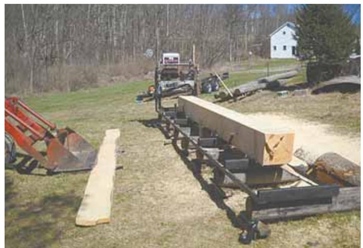
He used parts from a Sears Craftsman riding mower to build the sawmill, including the mower’s chassis and engine.
