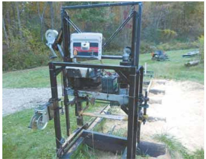
John Shultz turned his Stihl 046 chainsaw into this portable sawmill. But the only parts of the chainsaw he used were the 28-in. blade and sprocket.
