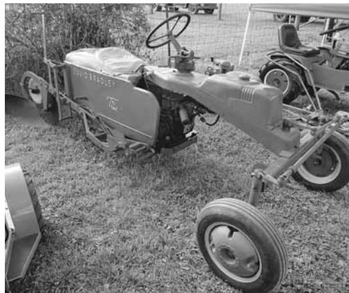
"The 3 wheels and long wheelbase made it tippy when turning, so the company tried to compensate by installing front wheel weights. The tractor didn't come with a differential. Instead, it has a forward and reverse variable speed transmission that works like a snowmobile clutch. Levers at the base of the steering column are used to control the clutch and throttle. Other levers are used to lift the plow and to adjust plow depth."
