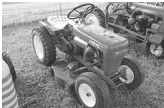
**1960 Wheelhorse Suburban 550.** The Suburban 550 was powered by a 5 hp Tecumseh engine and equipped with a 32-in. mower deck. Gittins's model still has the original tires. "The engine is located under the seat, and as a result it can get a little warm on your private parts," says Gittins.
