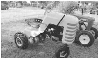
**1955 Sears Craftsman 3-wheeler.** Powered by a Craftsman 2 hp, 2-stroke Power Products engine, this tractor was originally designed to pull a reel mower. It weighs only 110 lbs. "This tractor doesn't have a reverse gear, but it's so light that you can push it backward with your feet as you're sitting down," says Gittins. "The operator uses a clutch lever connected to a belt tensioner to go forward. Brakes were optional. To stop, you put your feet down on the ground just like Fred Flintstone."
