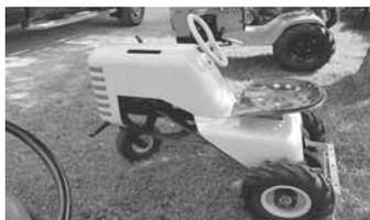
**1955 David Bradley Tri-Trac.** Unlike most 3-wheelers, the David Bradley Tri-Trac rides on 2 wide front wheels and a single rear wheel. It was designed to pull a 1-bottom moldboard plow. Power is supplied by a Wisconsin AKND 6hp engine. "This tractor wasn't particularly popular in its day," says Gittins. "The company built 3,000 AKND's, and it took 7 years to sell them all."
