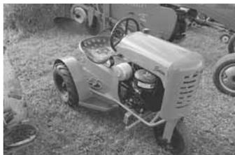
**1953 Bantam 14 3-wheeler.** The small Bantam 14 is powered by a 5 hp engine and belt-driven transmission and has a hand-operated clutch. "The cast iron steering wheel was unique to the Bantam," says Gittins.
