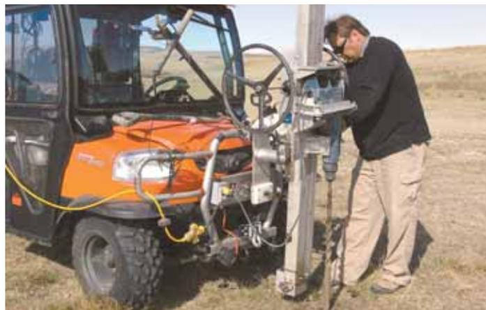
Gary Kehler uses seismoelectric technology to find water. He's shown here drilling a test shot hole with equipment mounted on his ATV.
