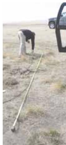
Sounding rods are driven into the ground about 15 ft. from the main hole. When a shotgun blast is fired into the hole, the seismic impact produces an electrical signal if water is present.
