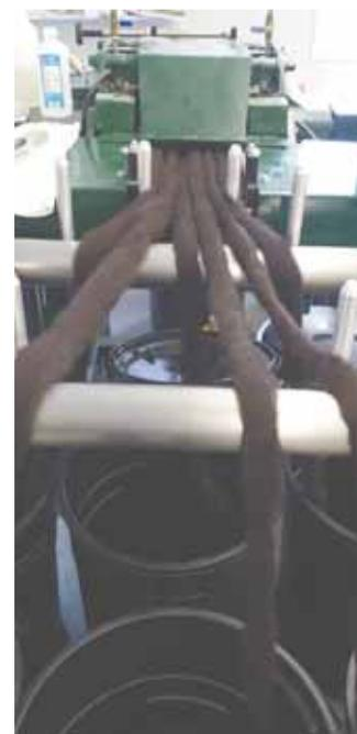
Their carding machine takes picked fibers and aligns them while removing dirt and foreign material.
