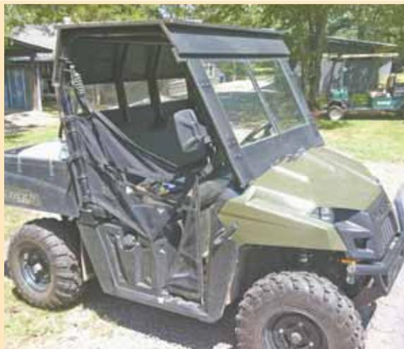
Glen King made a convertible cab for his Polaris UTV using 6 wooden panels that U-bolt to the rollover bars. "I can remove the entire cab in 20 min. or just take off pieces," he says.
