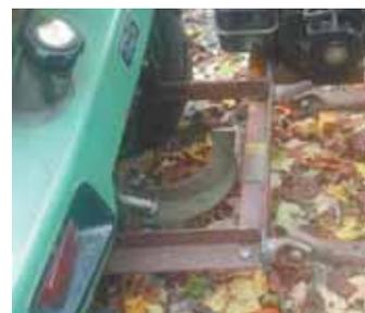
problem, I designed a hitch system that supports the motor and fastens to the vac with two 1/2-in. bolts and a 3/4-in. dia. hitch pin. The hitch pivots up and down and twists back and forth. All the metal came from an old hay rake, including the curved brace that connects with the hitch pin."
