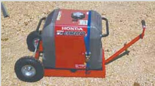
**Homemade generator cart rides on 10-in. pneumatic tires, allowing the cart to roll easily over uneven ground.**
