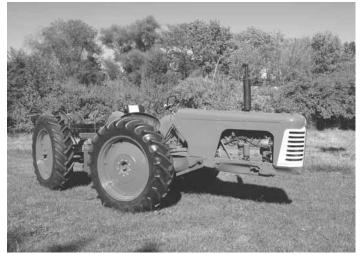
Ollie Schaefer can run his articulated Oliver 88 tractor with either front-wheel drive, The only real problem Schaefer has had is remembering which transmission is in gear. rear-wheel drive or 4-wheel drive.
